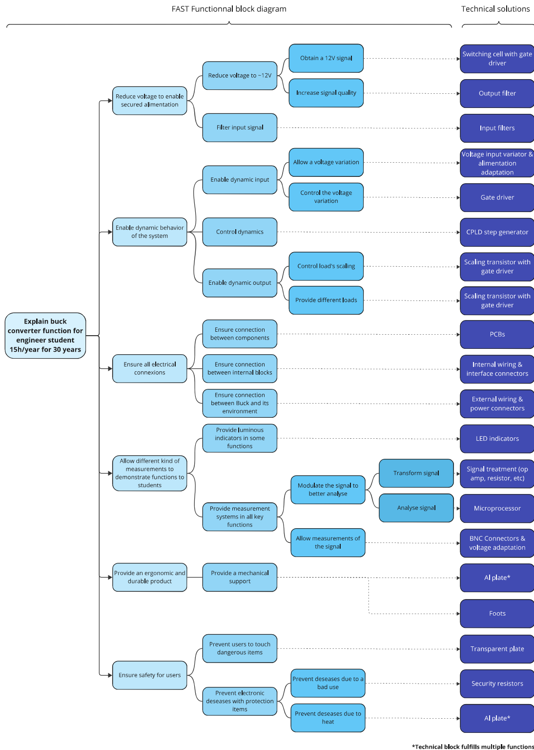
Figure 4.2-FAST diagram with functional structure of the buck converter [34]
