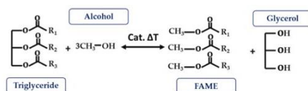
Fig. 2. Biodiesel production through transesterification reaction [5].
