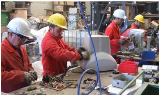
The processes for managing obsolete equipment are as follows. Once withdrawn from use, the televisions and monitors are transferred to a waste electrical and electronic equipment (WEEE) treatment plant, where they are subject to a number of processes for the removal and selection of certain materials, such as metals and plastics for their subsequent shipment to recycling companies. These processes
